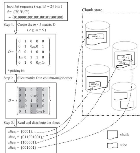
Fig. 3. An example of the bit-interleaving process
