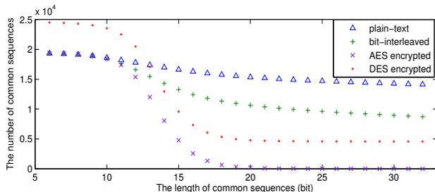
Fig. 8. Number of common bit sequences in two versions of the “/kernel/mutex.h” file in the Linux kernel
