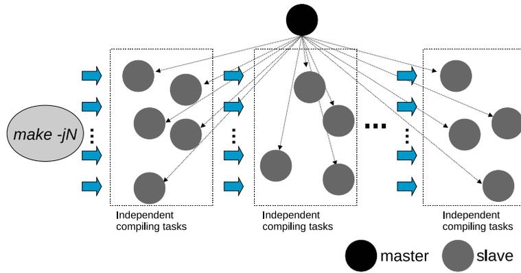
Figure 3.1: The architecture of mrcc
