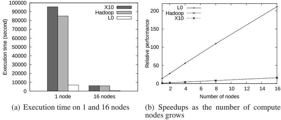
Figure 6.3: Execution time and speedups of  $k$ -means
