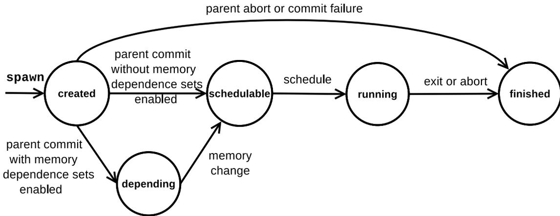
Figure 4.4: State transition of the task and depending task
