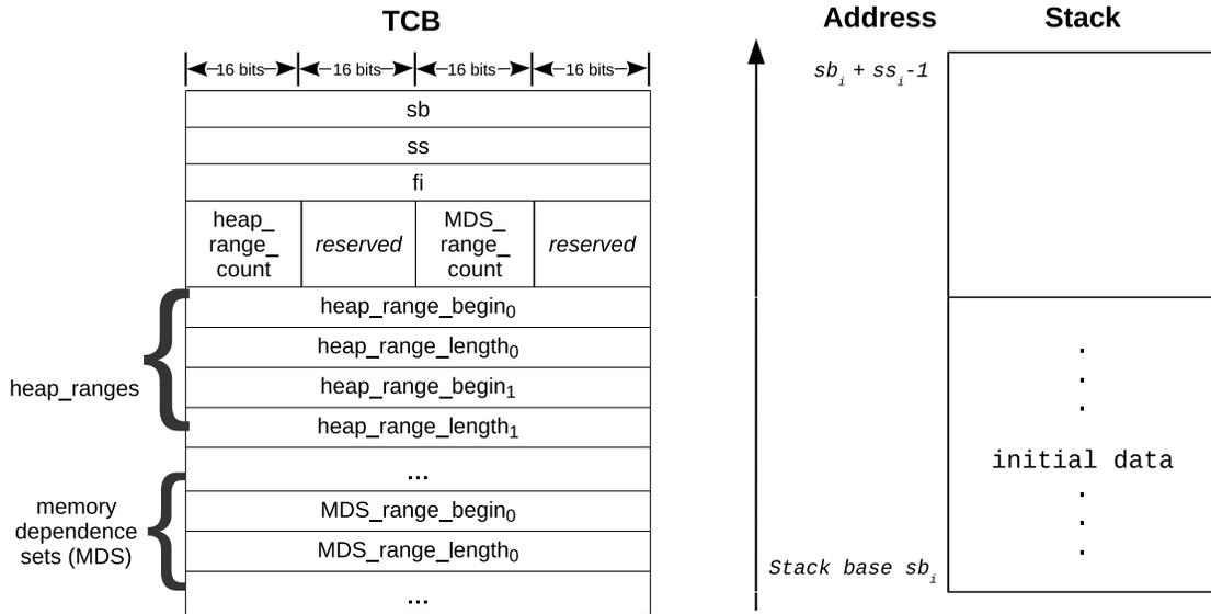
Figure 4.5: Task  $i$ 's initial stack and TCB
