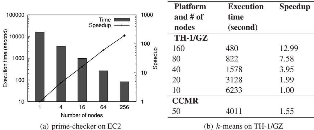
Figure 6.5: Scalability with the number of compute nodes
