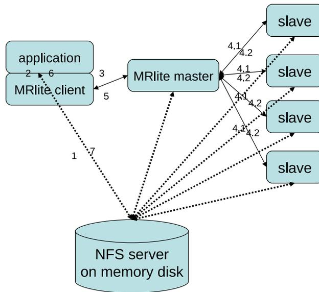
Figure 3.3: The architecture of MRlite
