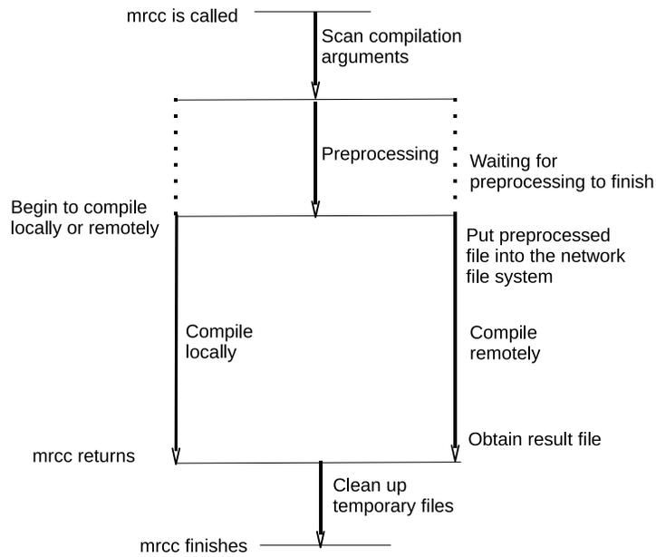
Figure 3.2: The work flow of mrcc
